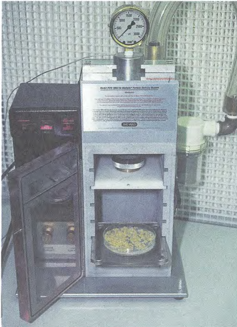
FIGURE 6A: The Biolistic ® Accell ® gene gun.
